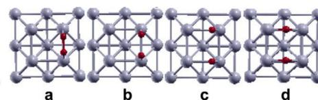
Fig.6: Selected states along the path of O<sub>2</sub> dissociation on Ir(100) surface and the reaction minimum energy path. Erikat (2011)
