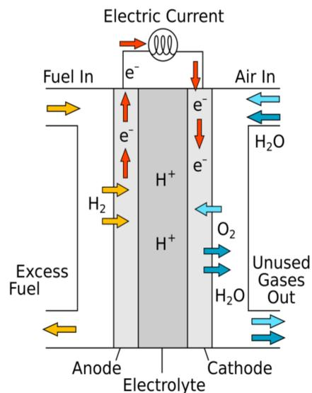
Fig.1: PEMFC schematic
