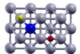
Fig.3: The high symmetry sites: yellow for top, blue for hollow and red for bridge
